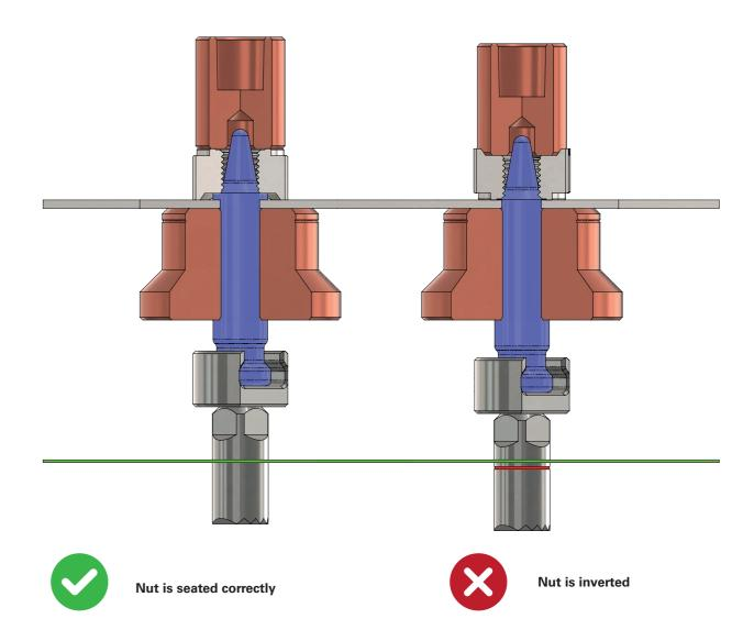
The sensor technology on the **ModulMaster** registers in real-time whether the centring pin is in the correct position for the respective welding process. This enhances the process reliability and quality assurance during production and significantly reduces waste.
